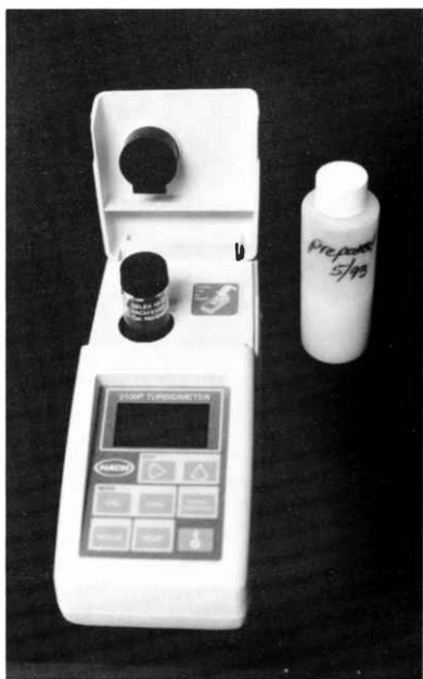
A portable turbidimeter measures turbidity.
