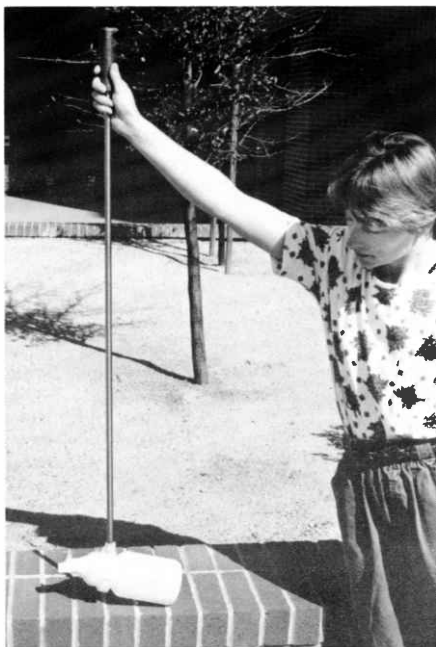
Grab samples of surface water can be collected with a DH-81 sampler (shown here with a stainless steel handle).
