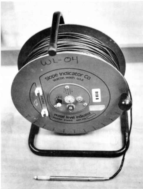
An electric sounder measures depth to water.
