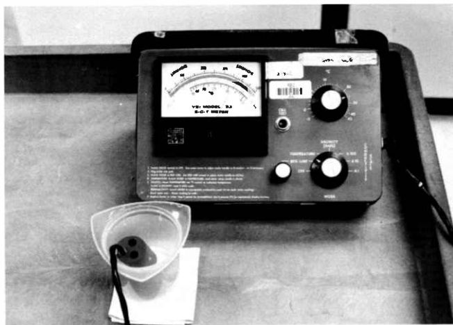
A temperature-pH-conductivity meter is used for measuring physical parameters of water in the field.
