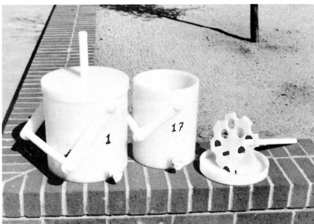
Churn splitters are used for compositing river samples.
