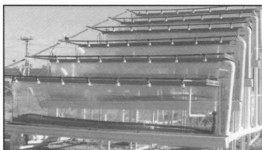
An outdoor multi-stage, continuous-flow photobioreactor (MCP) for groundwater nitrate removal.
