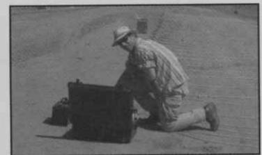
*Graduate student Andrew Hinnel was one of the UA students to receive a TRIF fellowship. He is shown making electrical resistance tomography measurements to track the movement of subsurface water.*
