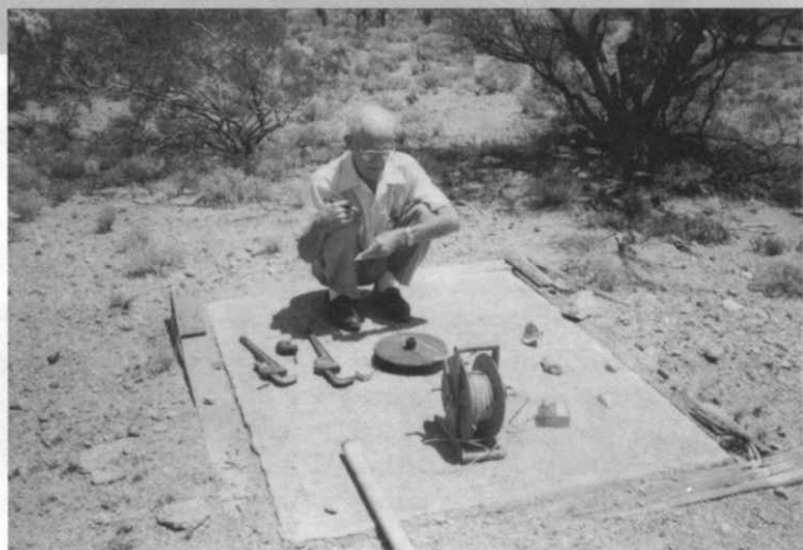
Leonard was active into his 80s. In this 1994 photo he uses a homemade sounder to measure water levels in a well. (Photo: Phil Halpenny)
