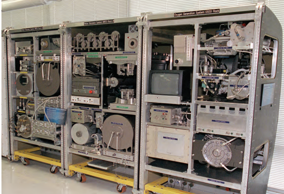
The Environmental Control and Life Support System Mockup for the International Space Station includes a Water Recovery System that uses an extensive filtering process. Source: NASA Marshall Space Flight Center
