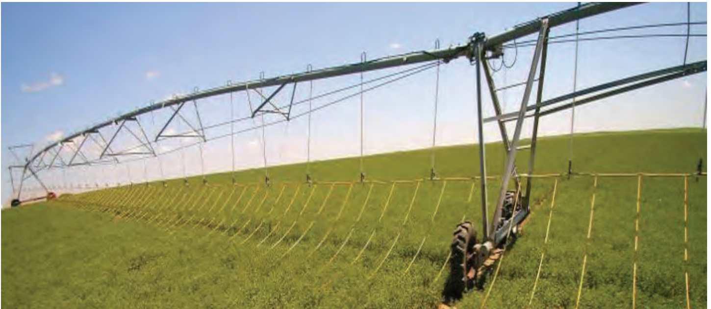
Center pivot sprinkler irrigation with drip lines is a water saving innovation. Image: https://img.agriexpo.online
