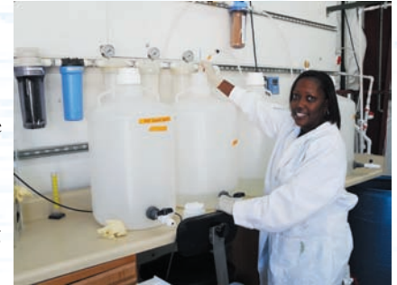
Miles in the Real-Time Monitoring Laboratory at the Environmental Research Laboratory filling a carboy with water that will be seeded with E. coli and passed through the lab’s field-scale distribution system.
